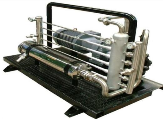
WyunaSep Hydrocyclone use centrifugal force to Physically separate fats or solids from water or water based solutions regardless of the flow rate.
